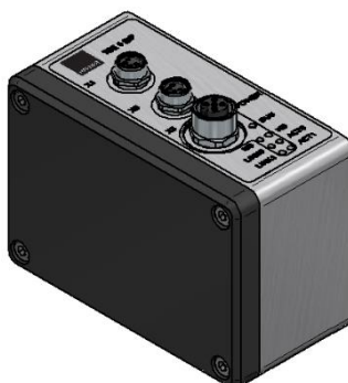
X0: Ethernet/IP IN: M8 4pin female
